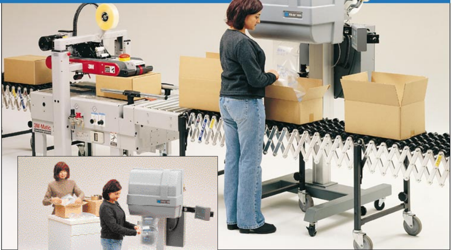
The versatile, highly productive Fill-Air™ system can be used on-line or to supply on-demand cushions for multiple packaging stations.
